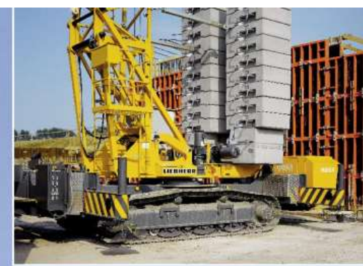
The 42 KR.1's compact crawler travel gear.
